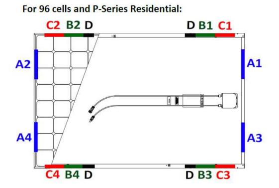
Design Load 2.4 kPa downforce 6.0 kPa downforce / / 2.4 kPa uplift 3.6 kPa uplift Clamp Zones B & C (mm)<sup>1</sup> 50-640 230-440 Clamp Width Requirements (mm) ≥ 35 Maximum Clamp Torque (for 120 in-lbs (13.5 Nm) flat/non-grounding clamp interface) Maximum Clamp Torque (for 50 in-lbs (5.6 Nm) serrated/grounding clamp interface)
