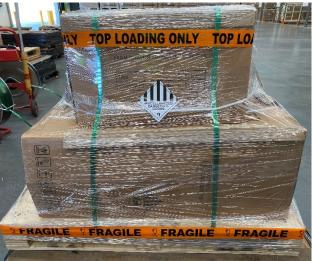
When shipping multiple units, same procedure should be utilized. Inverters can be restacked to the desired quantity in the same arrangement.
