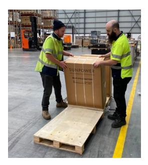
While utilizing minimum two people, adopt a stable position, get a good hold of the carton utilizing manufactured handgrips where possible, and carefully tilt the battery and take the weight so it does not fall onto the pallet / skid and ensure that the battery does not slip off the pallet / skid.
