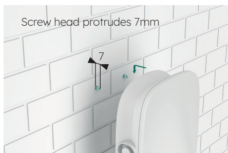
Figure 16 Hanging charging station
