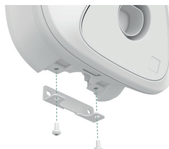
Figure 17 Fixing bottom of charging station
