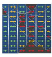
Figure 5: Not only are the smaller cells of the Performance panel less susceptible to breakage, but they confine cracks to a smaller portion of the panel, while maximising energy generation through a series of redundant electrical connections.
