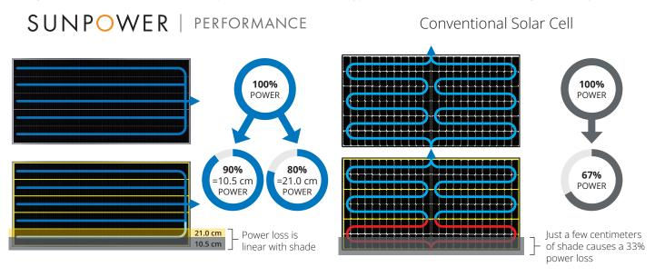
Figure 6: The parallel cell architecture of the Performance panel minimises power loss from shading and soiling in landscape orientation.
