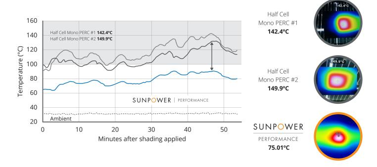
Figure 11: Under severe cell cracking or worst-case shading conditions, Performance panels operate at 40-50°C lower temperature, reducing the risk of temperature-related failures.9
