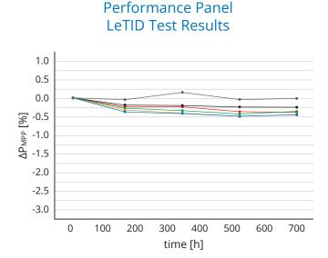
Figure 12: Fraunhofer LID and LeTID test results for Performance panels.
