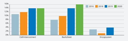
Figure 3: Inspection results from Dupont's Global PV Reliability Field Analysis featuring key causes of panel failure amongst recently installed conventional panels.
