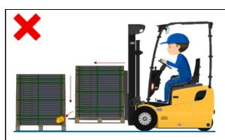
Ensure the forks **do not extend** beyond the pallet, as this can cause damage to the next pallet
