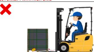
Make sure **not to tilt the fork up** while going through the pallet, doing so may impact the back sheet of the bottom modules or just cut the strapping
