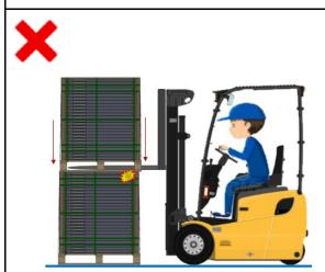
Double stack the pallet with care Gently place the top pallet on the border frame Ensure the forks do not hit the top module while taking them away
