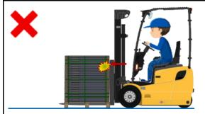
Ensure the backrest of the forklift does not hit the pallet
