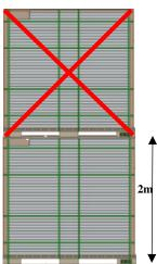
Triple stack is not allowed Double stack for 2 meters high pallets is not allowed
